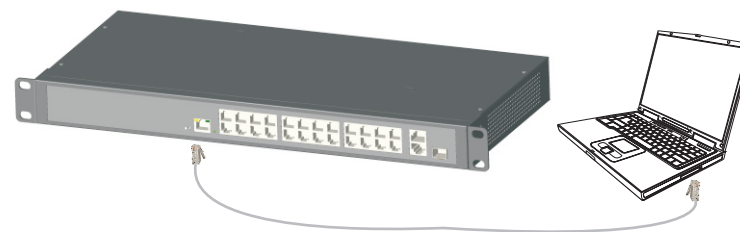
Figure 2-5 Connect configuration cable
