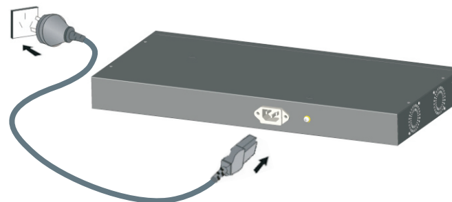
Figure 2-6 Power line connection
